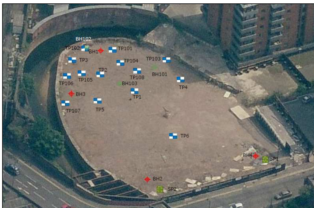
Plate 9: Location of the trial pits and boreholes
